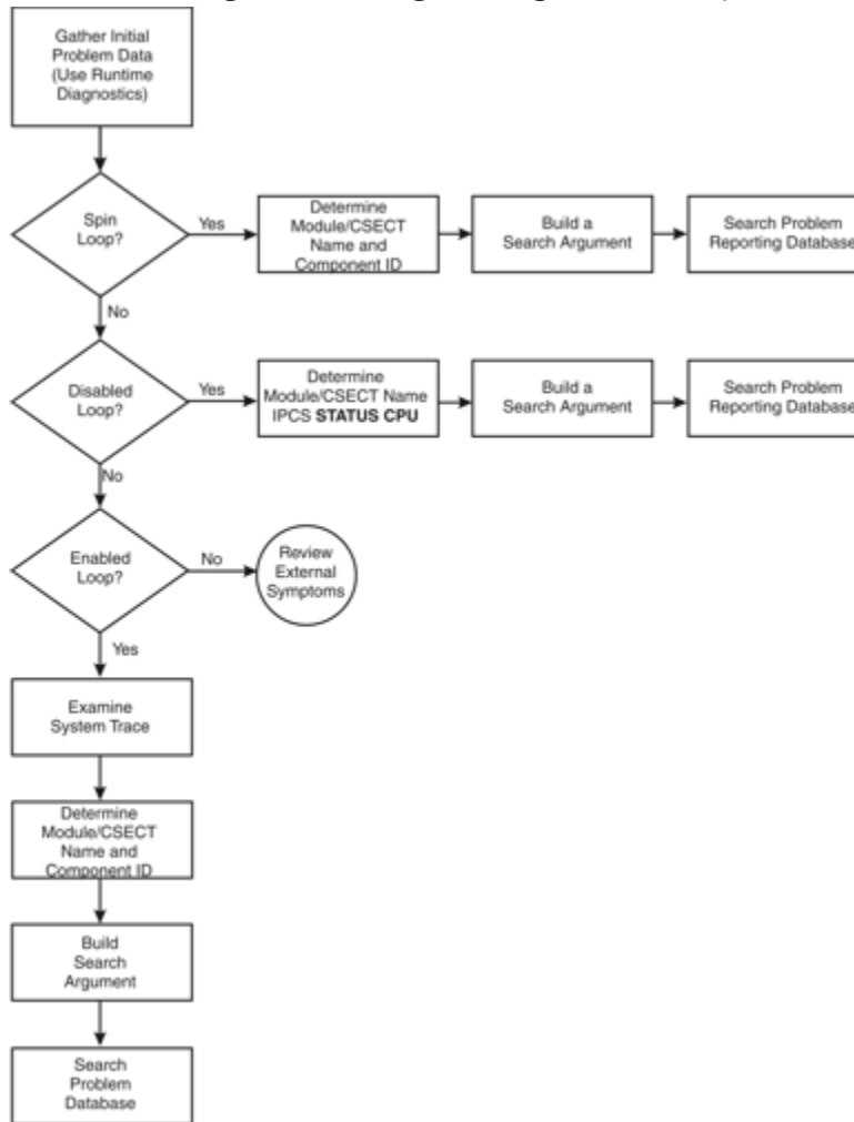
Figure 54. Flowchart for diagnosis of a loop
