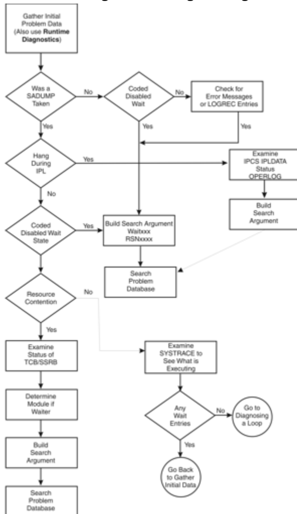
Figure 50. Flowchart for system hang analysis
