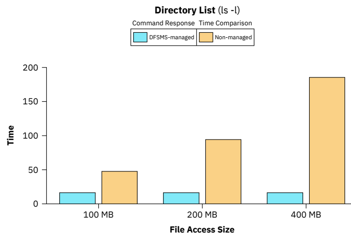
Figure 48. Directory list comparison between DFSMS-managed and non-managed
